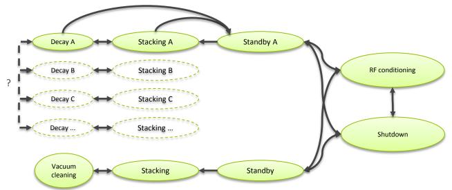
**Standby:** relevant magnet settings applied, RF on, valves open, IDs open (?), no beam **Stacking:** active injection kicker. Once current is above certain limits, activate feedback on orbit/tune/coupling/bbb, allow closed IDs (?). MPS switches on orbit interlocks over 5 mA.
