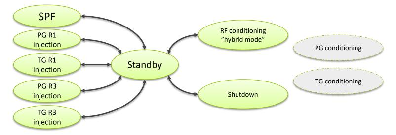
**Standby:** Mode with blocked/disabled beam, to allow machine changes in a safe way from PSS perspective.
