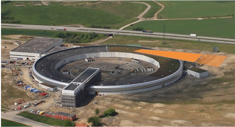
Figure 1.1. Aerial picture of the MAX IV facility under construction with depiction in orange where the SXL beamline would be located after the 3 GeV linear accelerator. In shaded orange is indicated future expansion possibilities.
