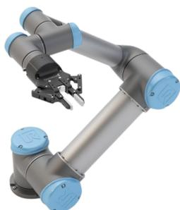
The system employs a Universal Robots UR10e robotic arm equipped with a RobotIQ 2F-85 gripper to automate the handling of catalyst samples. Each sample is secured within a glass capillary tube attached to a standardized holder, uniquely identified by a QR code. The QR code stores the sample holder ID which is linked to the sample ID, enabling seamless tracking throughout the experimental process.
