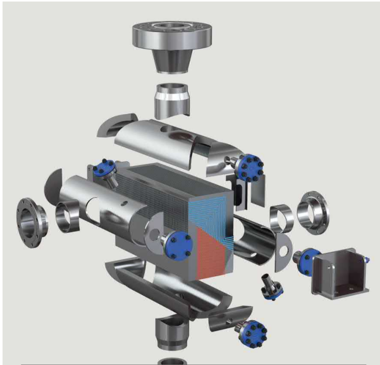
Alfa Laval Printed circuit heat exchangers product brochure : Stacked microchannel plates joined together by vacuum diffusion bonding
