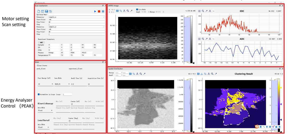
**Embedded clustering** algorithm for realtime segmentation of distinct electronicstructure regions on the sample surface.
