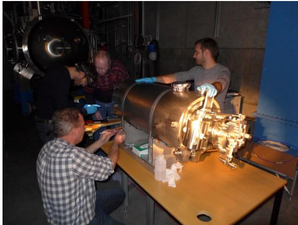
ESS086-P01 High- \beta elliptical cavity with FPC
